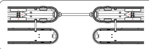
step6:4Fasten the waterproof connector from other end of the waterproof fitting and insert the wire into the terminal block. Using the same cable fasten the waterproof connector of the 2nd waterproof fitting and wire into the terminal block.
