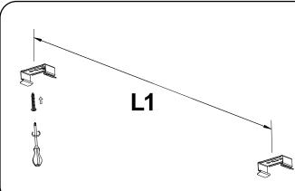
**STEP2:** Fix the mounting brackets onto the ceiling using screws and expansion plug(included). Please refer to table 1 for installing the mounting bracket distance points.
