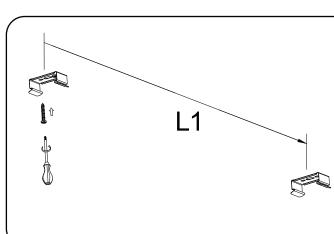
**STEP2:** Fix the mounting brackets onto the ceiling using screws and expansion plug(included). Please refer to table 1 for installing the mounting bracket distance points.
