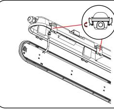
**STEP4:**4Open the side clips of water-proof fitting and open the diffuser as shown in the diagram.
