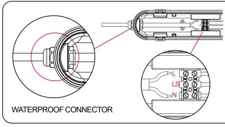
**STEP5:** Wiring 1stwaterproof fitting from both the ends - Fastenthe waterproof connector clockwise from the first end and insert the cable through the waterproof connector and wire into the terminal block from one end.
