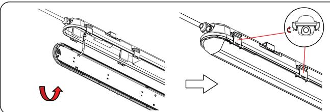
**STEP6:** Install the diffuser to the waterproof fitting and close the clips.
