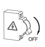
**STEP 1:** Switch OFF the power before starting the installation.
