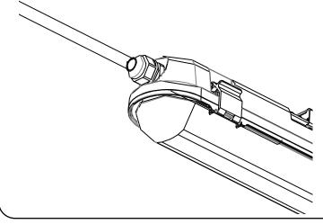
**STEP7:**4Wire the water-proof fitting to the main power supply. Ensure to use waterproof terminal block [not included].
