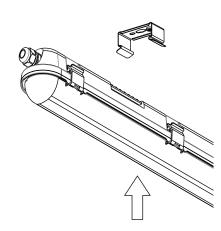
**STEP3:** Mount water-proof lamp onto the mounting brackets.
