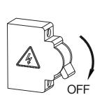
**STEP 1:** Switch OFF the power before starting the installation.
